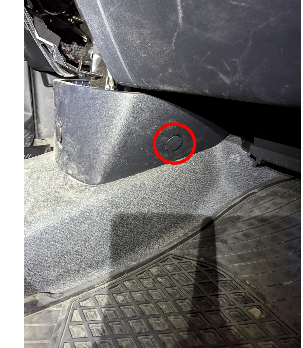
Loosen the 12V outlet connector by pulling it upwards.
