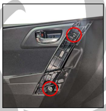
8. Remove the window switch panel
